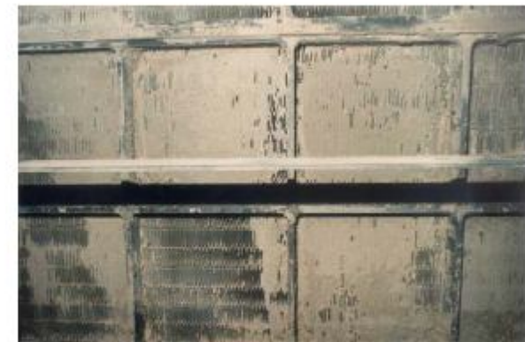
plugged plate-type catalyst
