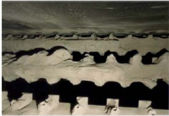
plugged NH 3 -injection system
